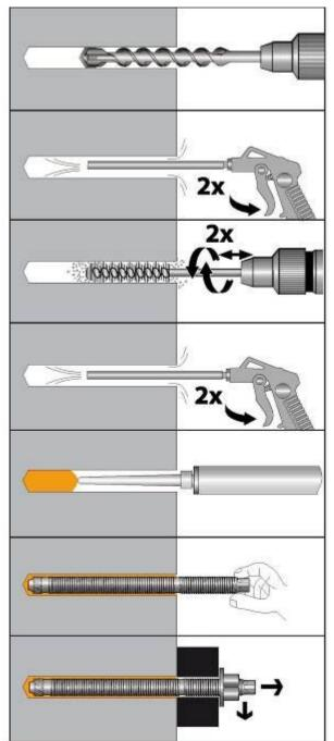
Drill hole of diameter ( $d_0$ ) and depth ( $h_0$ ) with a hammer drill set in rotation-hammer mode using an appropriately carbide drill bit.
