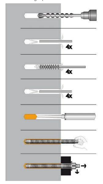
Drill hole of diameter  $(d_0)$  and depth  $(h_0)$  with a hammer drill set in rotation-hammer mode using an appropriately carbide drill bit.
